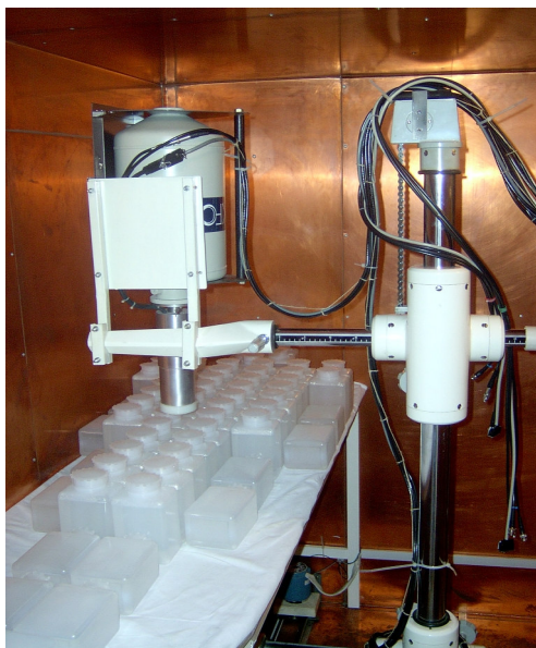
Fig.5. Calibration of human Whole-Body Counter (gamma-spectrometer) using a "flask-phantom"
