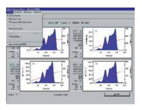
The Model 8800 is controlled through screen dialogues, using the mouse to make selections from the drop-down menus. It can also be networked with Model 4500 and Model 6600 in discrete or shared dosimetry applications.
